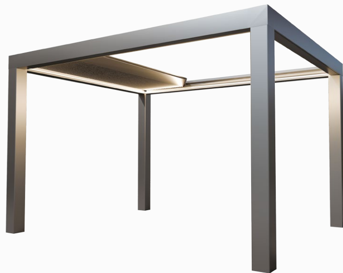
HF228 Retractable Louvered Pergola ▪ Max size: Width 4m * Extend 6m (width can be infinitely spliced) ▪ Frame: 6063-T5 Aluminum Alloy ▪ Optional: LED light strip, Zip screen blinds
